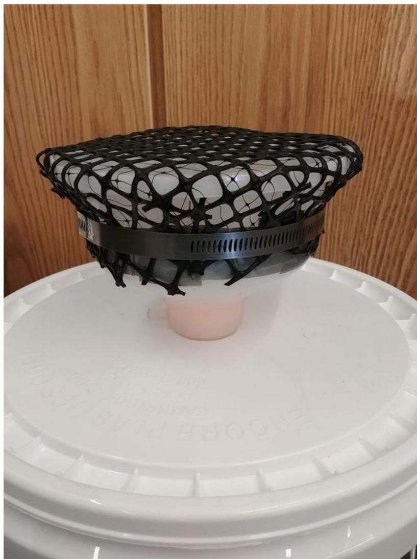
**Figure 12. Precipitation collectors.** Water passes through the plastic mesh and past the buoyant ping-pong ball to the 4-liter jug nested inside the bucket.
